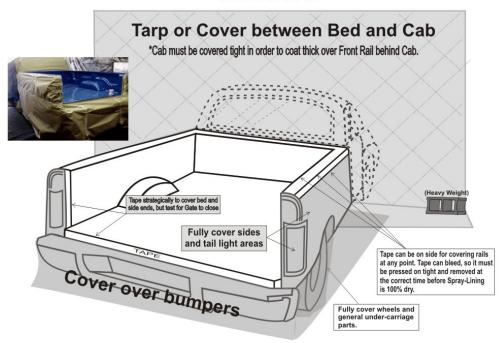
\* All tape & covers (tarps, paper or plastic) must adhere to each other & truck parts 100% with 0% openings or leaks. \*Tape at exact, well thought out points for Spray-Lining to provide maximum protection.
